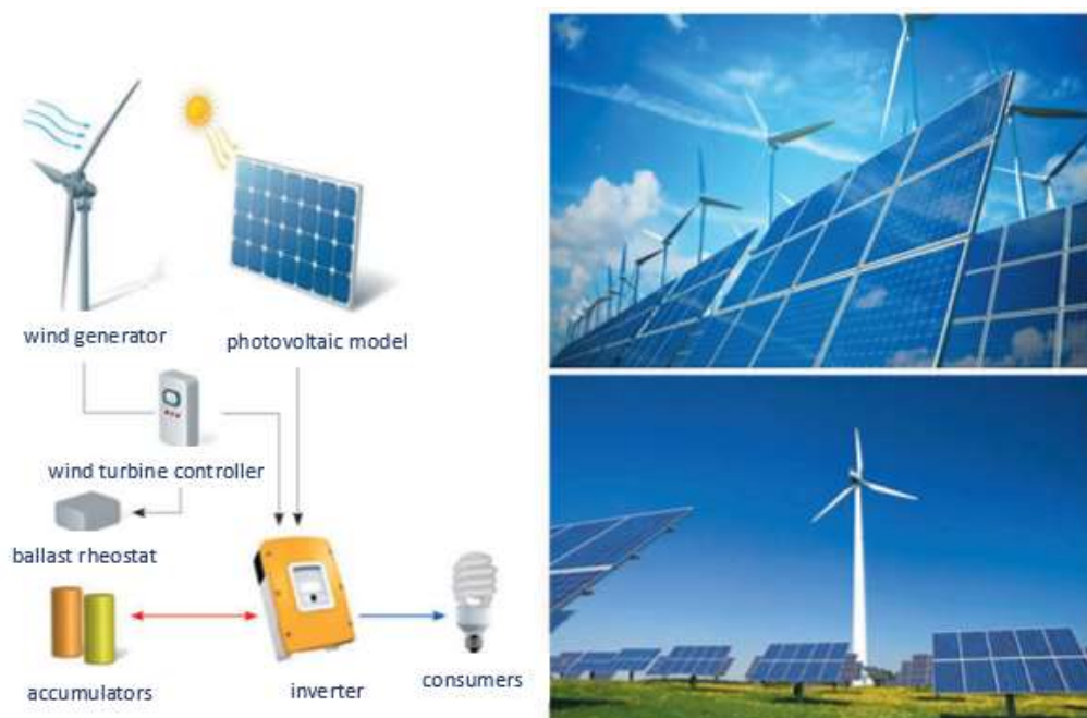
Fig.1 1. Conventional diagram and appearance of a wind-solar power plant (wind power plant)
